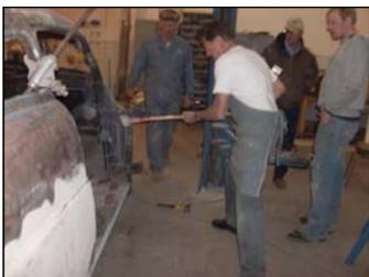
*Gene Winfield demonstrates how to adjust the door hinges on a '50 Mercury by swinging a sledge hammer.*
